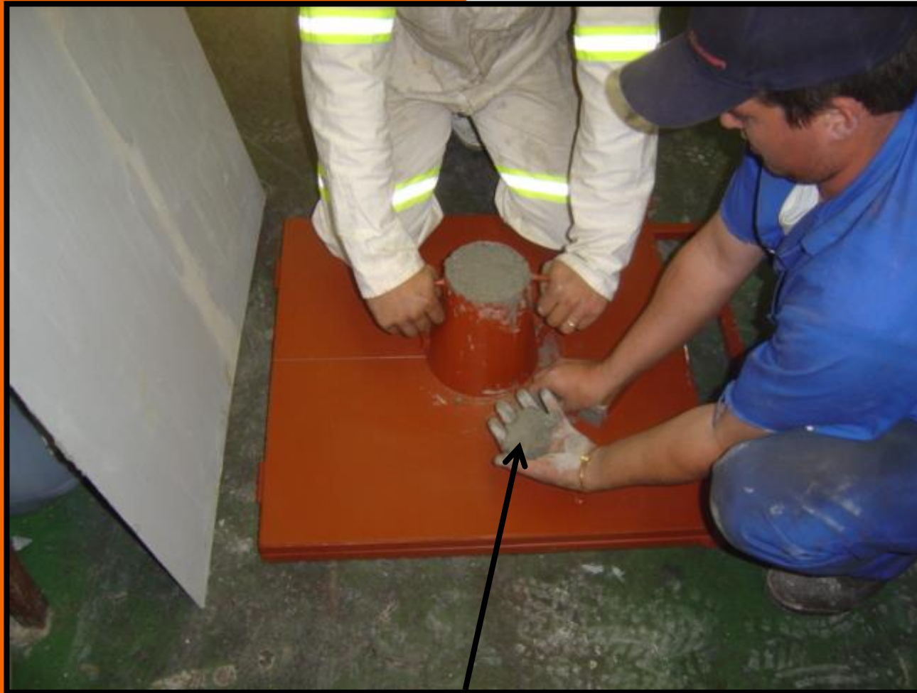
Clean Flow Table Spillage
