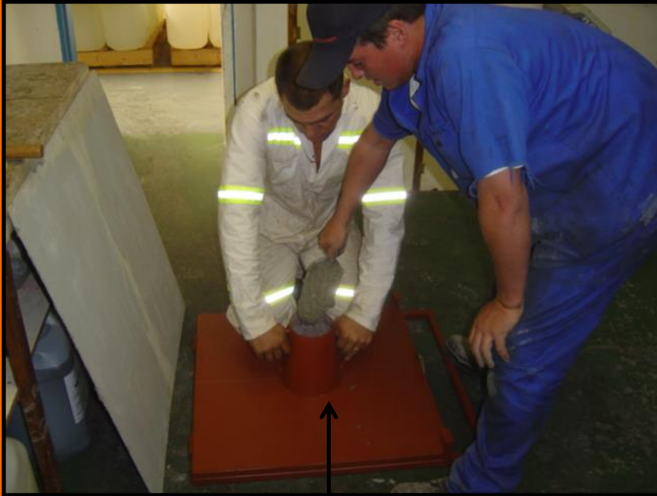
Half Fill Flow Cone
